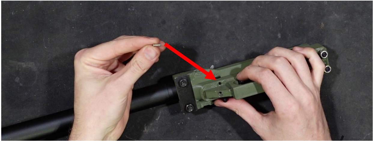
Insert the detent into its hole.
