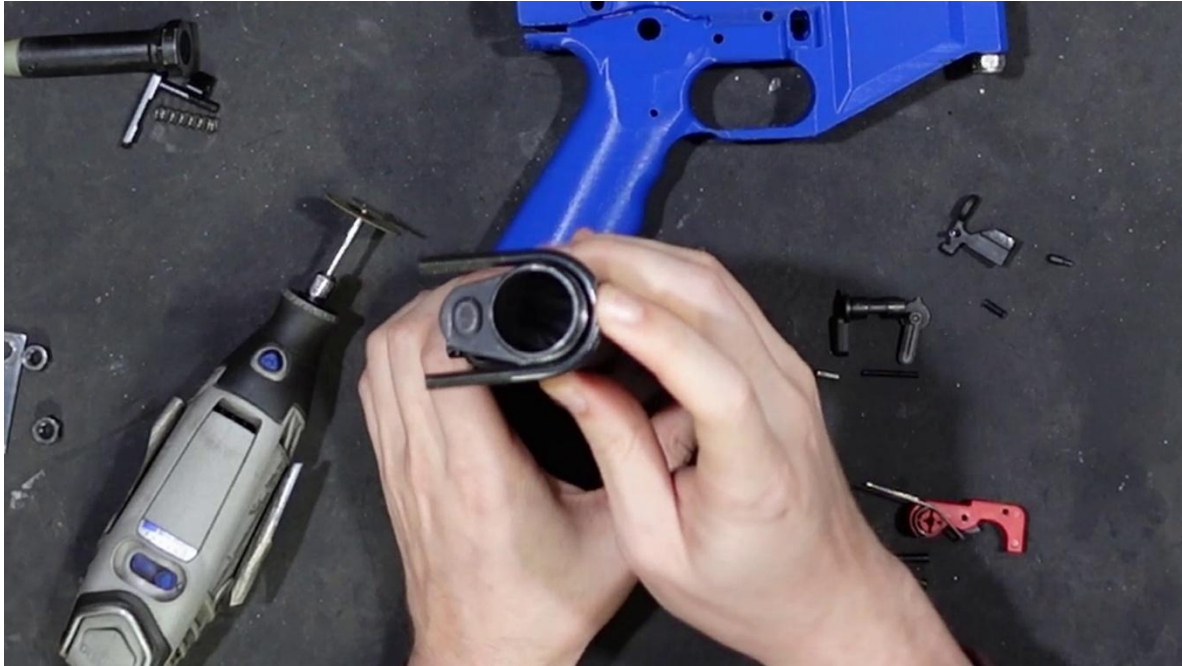
First, make sure the u-bolt fits down over the buffer tube.
