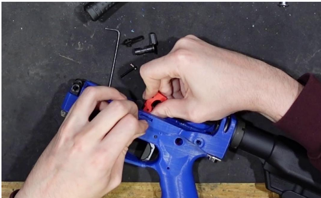
Install the hammer – again, just like a standard AR15 build.
