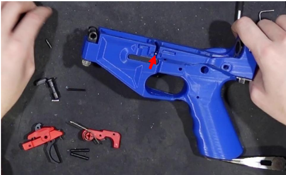
View of the installed detent and spring
