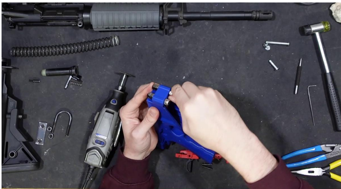
Secure the eyebolts with a pair of nuts. Do not tighten these nuts all the way, leave them loose so that the eyebolts have a little wiggle. We will tighten them after the upper is installed.
