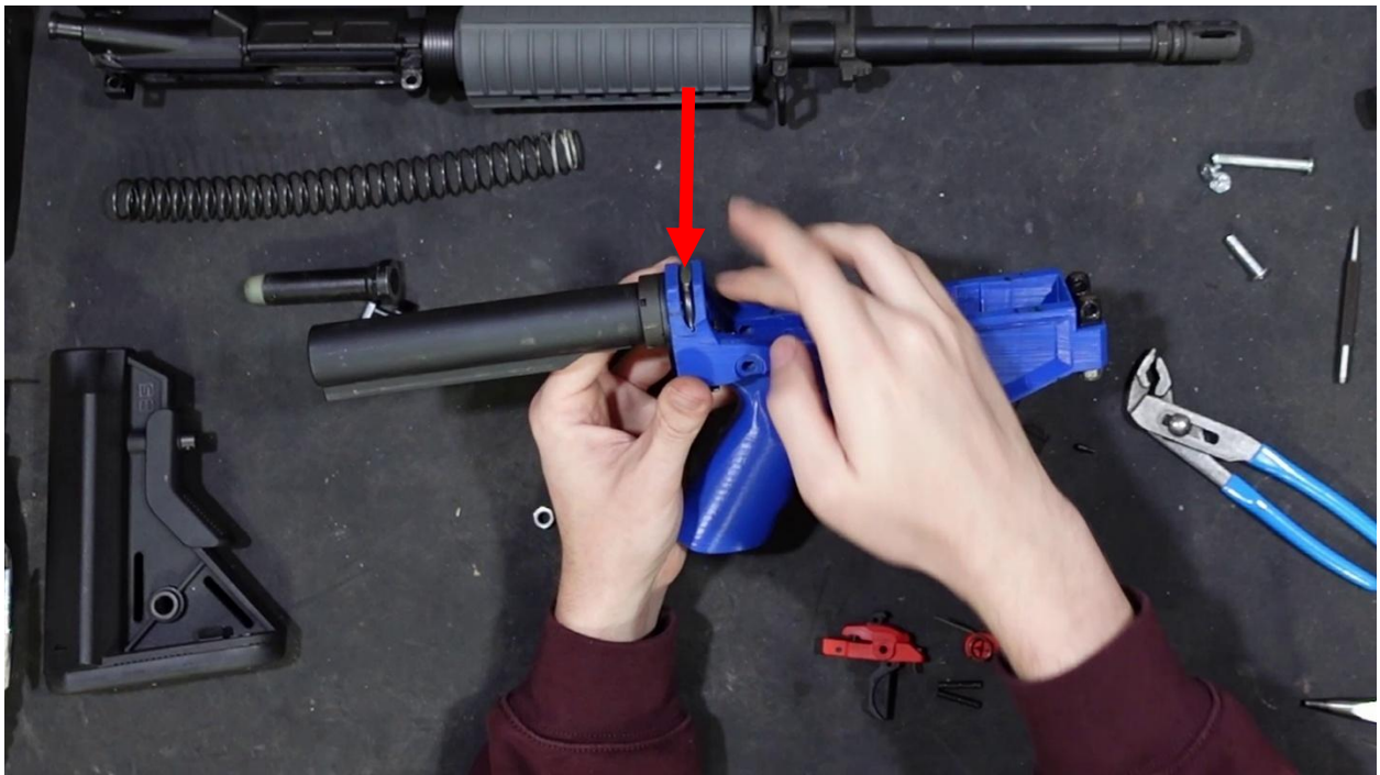
Make sure that the top of the u-bolt is ground down so that it sits flush (or slightly below) the top of the buffer tower. Refer to Step 2 for instructions on this. Do not grind on the u-bolt while it is installed in the lower!
