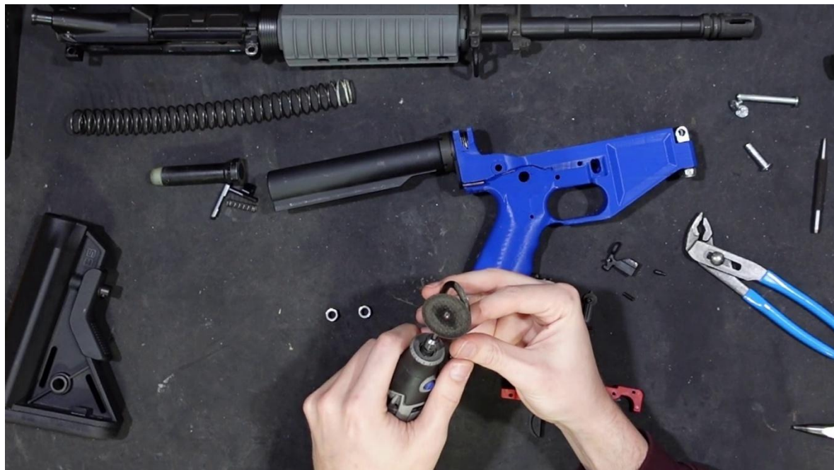
Then use a Dremel or hand file to remove material off the top of the u-bolt so that it sits flush with the top of the lower. NOTE: I recommend you install the buffer tube first before doing this. Refer to Step 4.
