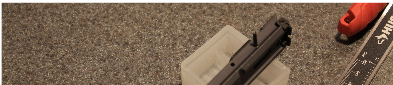
Place the pin in, then use the 4mm pin punch to send it home.
