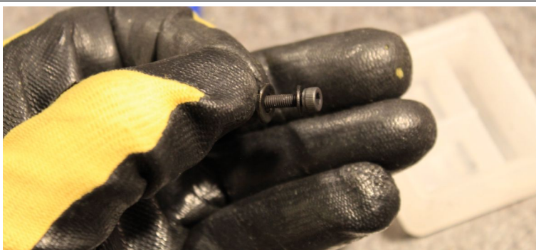
M3 bolt with an M3 washer and M4 washer
