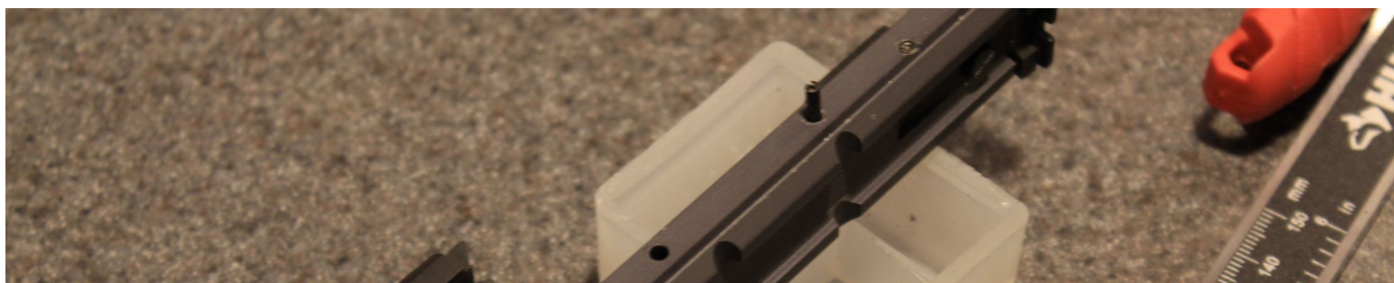
The pin should be slightly flush on both sides, so switch to the 2mm punch and give the pin a small tap to make it just below the side you're going in from. It should be below the rail surface on both sides when done. Repeat for the other 2 pins.
